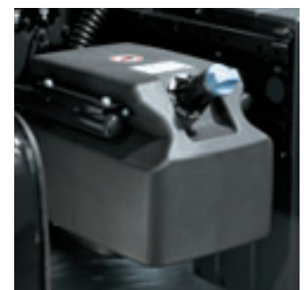
Separate AdBlue ® tank for construction vehicles.
