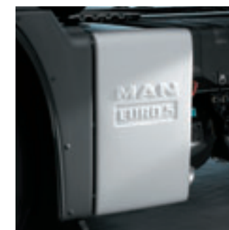
Silencer with SCR catalyst for Euro 5.
