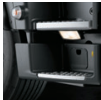
Manoeuvring light in the co-driver's entry.
