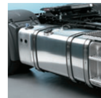
Combined tank for diesel and AdBlue ® .
