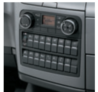
New controls for the air conditioner, heater and ventilation. New switch field with function displays.
