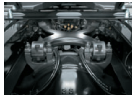
Weight-optimised X control arm with a stabiliser and steering function for semitrailer tractors and high-load roll stabilisation.
