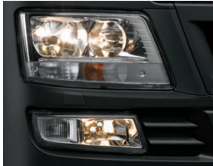
Headlights with free-form reflectors, Xenon dipped headlight.
